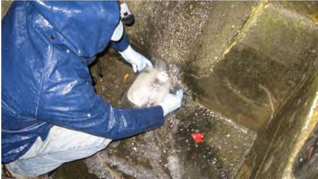
Collecting a sheet flow stormwater sample.
